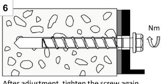
After adjustment, tighten the screw again
